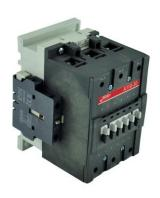
PART NUMBER – BA110-30-11-81: BRAH Electric, aftermarket direct replacement contactors for ABB A110-30-11-81, A-Line series, type A, 3P, 3PH, 110A, 600V, 40HP @ 240V, 75HP @ 480V, 100HP @ 600V, complete with 24V AC coil, and 1 N/O - 1 N/C auxiliary contact, AC magnetic contactor, suitable for use with A-Line series motor control systems
