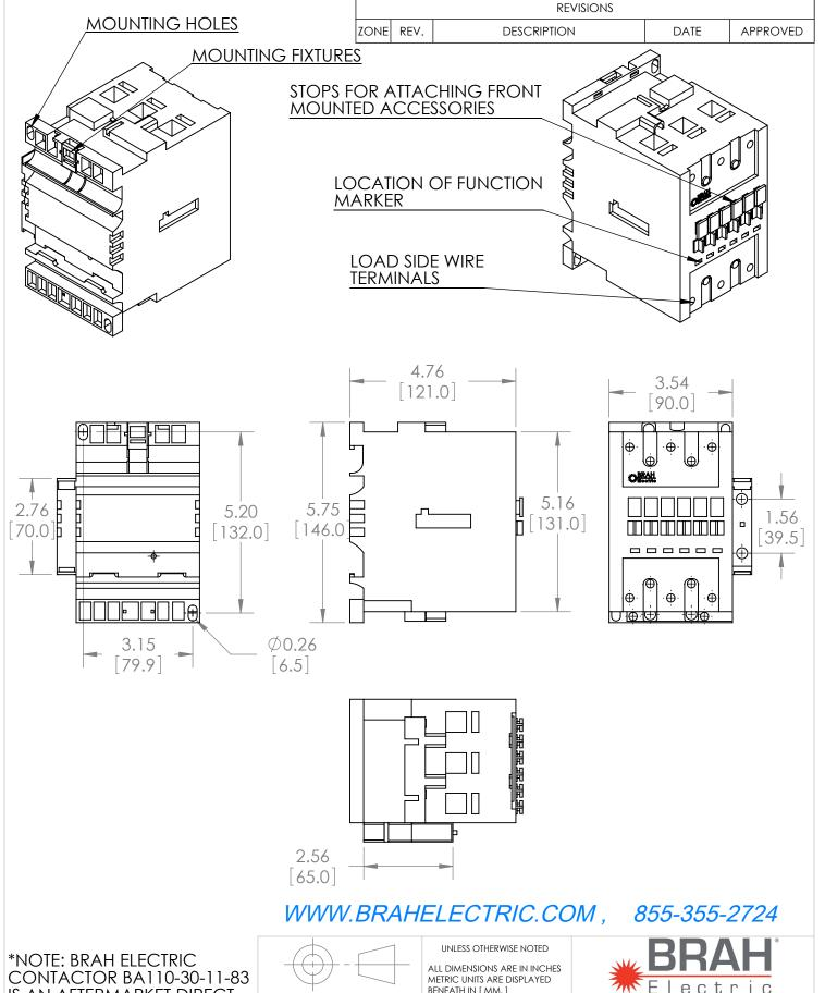
IS AN AFTERMARKET DIRECT REPLACMENT FOR A110-30-11-83, A-LINE SERIES. SUITABLE FOR USE WITH A-LINE SERIES MOTOR CONTROL **SYSTEMS**
