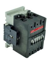
PART NUMBER – BA110-30-11-83: BRAH Electric, aftermarket direct replacement contactors for ABB A110-30-11-83, A-Line series, type A, 3P, 3PH, 110A, 600V, 40HP @ 240V, 75HP @ 480V, 100HP @ 600V, complete with 48V AC coil, and 1 N/O - 1 N/C auxiliary contact, AC magnetic contactor, suitable for use with A-Line series motor control systems
