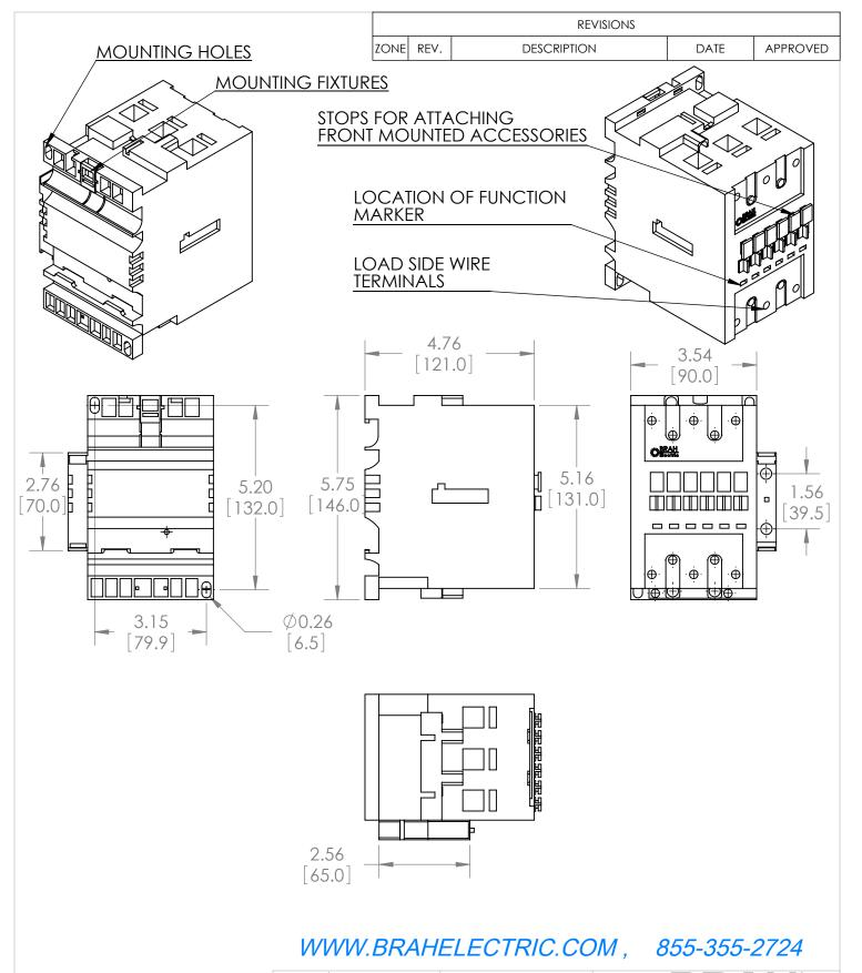
\*NOTE: BRAH ELECTRIC CONTACTOR BA110-30-11-86 IS AN AFTERMARKET DIRECT REPLACMENT FOR A110-30-11-86,A-LINE SERIES. SUITABLE FOR USE WITH A-LINE SERIES MOTOR CONTROL SYSTEMS
