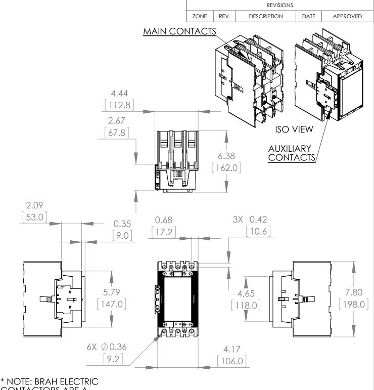
\* NOTE: BRAH ELECTRIC **CONTACTORS ARE A** DIRECT REPLACEMENT FOR ABB A145-30-11-51, A-LINE SERIES, TYPE BA, 3P, 3PH, 130A, 600V, 50HP @ 240V, 100HP @ 480V, 125HP @ 600V, COMPLETE WITH 480V AC COIL, AND 1 N/O - 1 N/C AUXILIARY CONTACT, AC MAGNETIC CONTACTOR, SUITABLE FOR USE WITH A-LINE SERIES MOTOR CONTROL SYSTEMS
