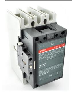
PART NUMBER – BA145-30-11-55: BRAH Electric, aftermarket direct replacement contactors for ABB A145-30-11-55, A-Line series, type A, 3P, 3PH, 130A, 600V, 50HP @ 240V, 100HP @ 480V, 125HP @ 600V, complete with 500/600V AC coil, and 1 NO/NC auxiliary contact, AC magnetic contactor, suitable for use with A-Line series motor control systems
