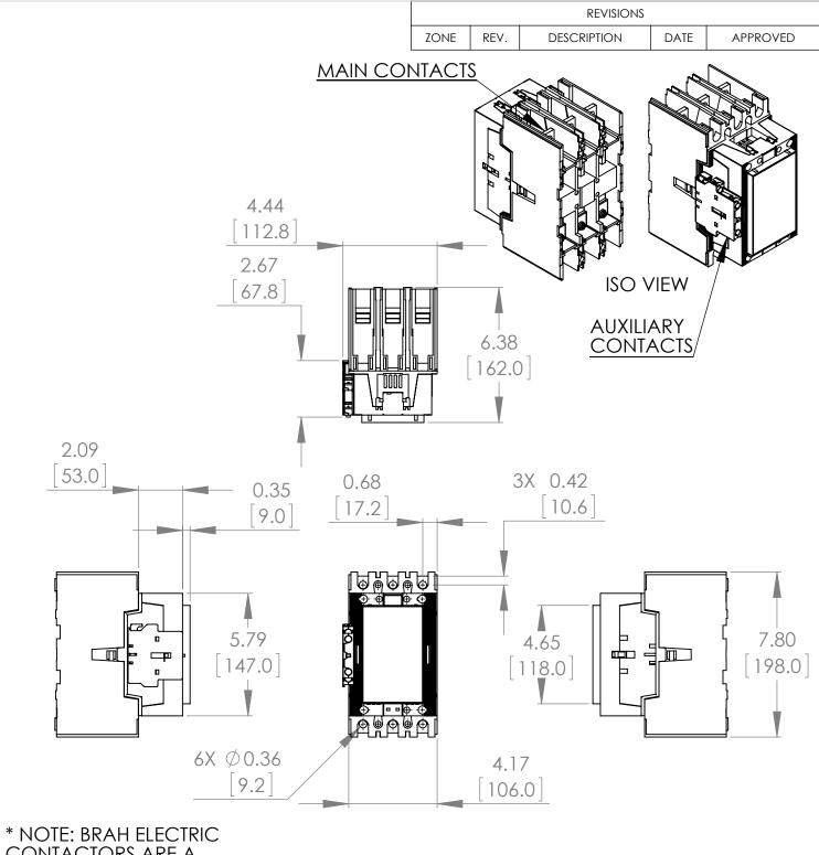
**CONTACTORS ARE A** DIRECT REPLACEMENT FOR ABB A145-30-11-80, A-LINE SERIES, TYPE BA, 3P, 3PH, 130A, 600V, 50HP @ 240V, 100HP @ 480V, 125HP @ 600V, COMPLETE WITH 220/240V AC COIL, AND 1 N/O - 1 N/C AUXILIARY CONTACT, AC MAGNETIC CONTACTOR, SUITABLE FOR USE WITH A-LINE SERIES MOTOR CONTROL SYSTEMS
