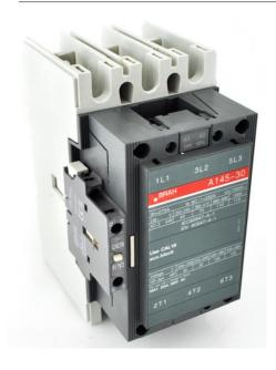
PART NUMBER – BA145-30-11-80: BRAH Electric, aftermarket direct replacement contactors for ABB A145-30-11-80, A-Line series, type A, 3P, 3PH, 130A, 600V, 50HP @ 240V, 100HP @ 480V, 125HP @ 600V, complete with 220/240V AC coil, and 1 NO/NC auxiliary contact, AC magnetic contactor, suitable for use with A-Line series motor control systems
