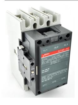
PART NUMBER – BA145-30-11-83: BRAH Electric, aftermarket direct replacement contactors for ABB A145-30-11-83, A-Line series, type A, 3P, 3PH, 130A, 600V, 50HP @ 240V, 100HP @ 480V, 125HP @ 600V, complete with 48V AC coil, and 1 NO/NC auxiliary contact, AC magnetic contactor, suitable for use with A-Line series motor control systems
