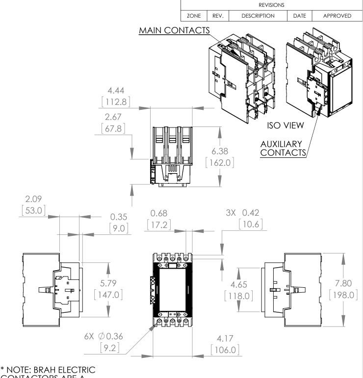
\* NOTE: BRAH ELECTRIC CONTACTORS ARE A DIRECT REPLACEMENT FOR ABB A145-30-11-84, A-LINE SERIES, TYPE BA, 3P, 3PH, 130A, 600V, 50HP @ 240V, 100HP @ 480V, 125HP @ 600V, COMPLETE WITH 120V AC COIL, AND 1 N/O - 1 N/C AUXILIARY CONTACT, AC MAGNETIC CONTACTOR, SUITABLE FOR USE WITH A-LINE SERIES MOTOR CONTROL SYSTEMS
