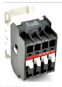
PART NUMBER – BA16-30-10-83: BRAH Electric, aftermarket direct replacement contactors for ABB A16-30-10-83, A-Line series, type A, 3P, 3PH, 17A, 600V, 5HP @ 240V, 10HP @ 480V, 15HP @ 600V, complete with 48V AC coil, and 1 N/O auxiliary contact, AC magnetic contactor, suitable for use with A-Line series motor control systems
