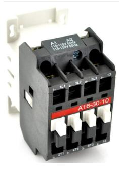
**PART NUMBER – BA16-30-10-86:** BRAH Electric, aftermarket direct replacement contactors for ABB A16-30-10-86, A-Line series, type A, 3P, 3PH, 17A, 600V, 5HP @ 240V, 10HP @ 480V, 15HP @ 600V, complete with 415/440V AC coil, and 1 N/O auxiliary contact, AC magnetic contactor, suitable for use with A-Line series motor control systems
