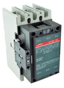
PART NUMBER – BA185-30-11: BRAH Electric, aftermarket direct replacement contactors for ABB A185-30-11, A-Line series, type A, 3P, 3PH, 156A, 600V, 60HP @ 240V, 125HP @ 480V, 150HP @ 600V, complete with 120V AC coil, and 1 NO/NC auxiliary contact, AC magnetic contactor, suitable for use with A-Line series motor control systems
