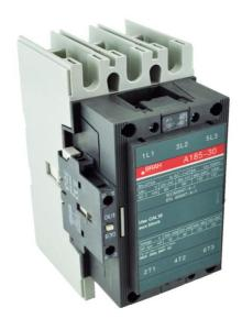
PART NUMBER – BA185-30-11-55: BRAH Electric, aftermarket direct replacement contactors for ABB A185-30-11-55, A-Line series, type A, 3P, 3PH, 156A, 600V, 60HP @ 240V, 125HP @ 480V, 150HP @ 600V, complete with 500V/600V AC coil, and 1 NO/NC auxiliary contact, AC magnetic contactor, suitable for use with A-Line series motor control systems
