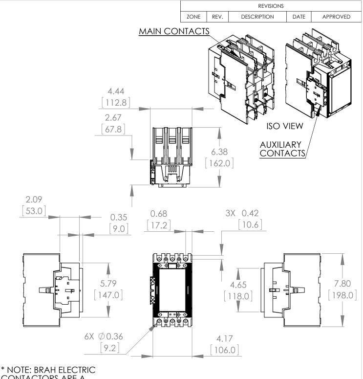
CONTACTORS ARE A DIRECT REPLACEMENT FOR ABB A185-30-11-55, A-LINE SERIES, TYPE BA, 3P, 3PH, 156A, 600V, 60HP @ 240V, 125HP @ 480V, 150HP @ 600V, COMPLETE WITH 500/600V AC COIL, AND 1 N/O - 1 N/C AUXILIARY CONTACT, AC MAGNETIC CONTACTOR, SUITABLE FOR USE WITH A-LINE SERIES MOTOR CONTROL SYSTEMS
