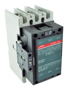
PART NUMBER – BA185-30-11-83: BRAH Electric, aftermarket direct replacement contactors for ABB A185-30-11-83, A-Line series, type A, 3P, 3PH, 156A, 600V, 60HP @ 240V, 125HP @ 480V, 150HP @ 600V, complete with 48V AC coil, and 1 NO/NC auxiliary contact, AC magnetic contactor, suitable for use with A-Line series motor control systems
