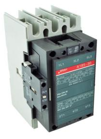
PART NUMBER – BA185-30-11-84: BRAH Electric, aftermarket direct replacement contactors for ABB A185-30-11-84, A-Line series, type A, 3P, 3PH, 156A, 600V, 60HP @ 240V, 125HP @ 480V, 150HP @ 600V, complete with 120V AC coil, and 1 NO/NC auxiliary contact, AC magnetic contactor, suitable for use with A-Line series motor control systems
