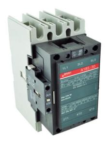
PART NUMBER – BA185-30-11-86: BRAH Electric, aftermarket direct replacement contactors for ABB A185-30-11-86, A-Line series, type A, 3P, 3PH, 156A, 600V, 60HP @ 240V, 125HP @ 480V, 150HP @ 600V, complete with 415/440V AC coil, and 1 NO/NC auxiliary contact, AC magnetic contactor, suitable for use with A-Line series motor control systems
