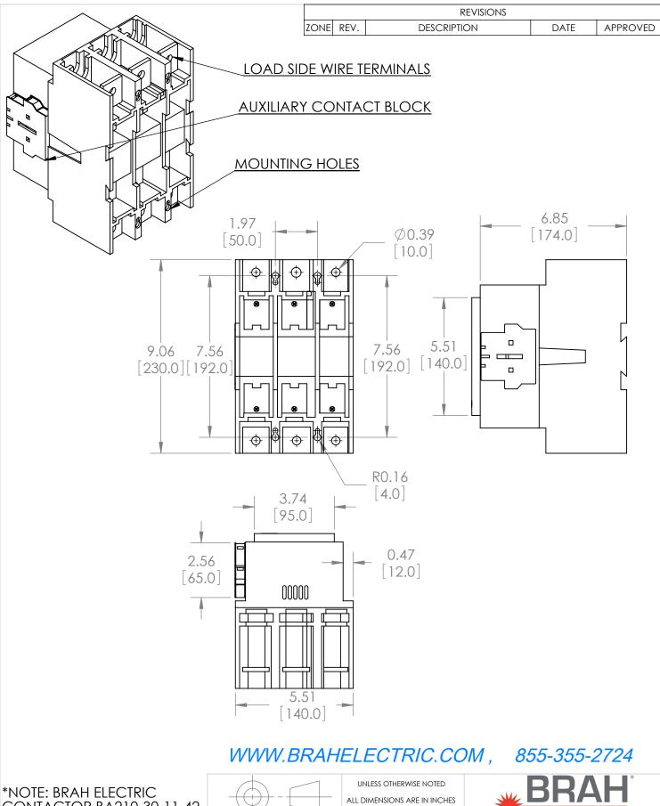
CONTACTOR BA210-30-11-42 IS AN AFTERMARKET DIRECT REPLACMENT FOR A210-30-11-42, A-LINE SERIES. SUITABLE FOR USE WITH A-LINE SERIES MOTOR CONTROL SYSTEMS
