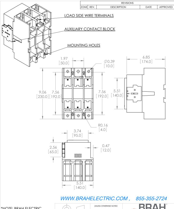
\*NOTE: BRAH ELECTRIC CONTACTOR BA210-30-11-80 IS AN AFTERMARKET DIRECT REPLACMENT FOR A210-30-11-80, A-LINE SERIES. SUITABLE FOR USE WITH A-LINE SERIES MOTOR CONTROL SYSTEMS
