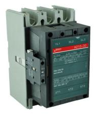
PART NUMBER – BA210-30-11-80: BRAH Electric, aftermarket direct replacement contactors for ABB A210-30-11-80, A-Line series, type A, 3P, 3PH, 192A, 600V, 75HP @ 240V, 150HP @ 480V, 200HP @ 600V, complete with 220/240V AC coil, and 1 N/O - 1 N/C auxiliary contact, AC magnetic contactor, suitable for use with A-Line series motor control systems
