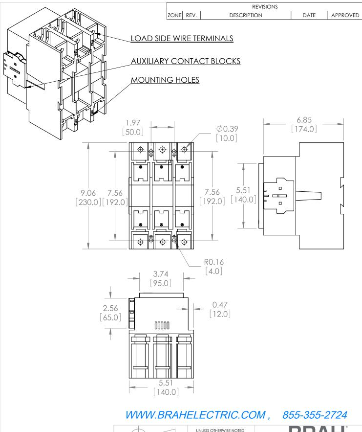
**\*NOTE: BRAH ELECTRIC** CONTACTOR BA210-30-11-83 IS AN AFTERMARKET DIRECT REPLACMENT FOR A210-30-11-83, A-LINE SERIES. SUITABLE FOR USE WITH A-LINE SERIES MOTOR CONTROL SYSTEMS
