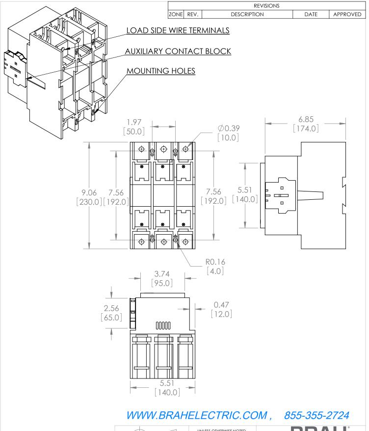
\*NOTE: BRAH ELECTRIC CONTACTOR BA210-30-11-84 IS AN AFTERMARKET DIRECT REPLACMENT FOR A210-30-11-84, A-LINE SERIES. SUITABLE FOR USE WITH A-LINE SERIES MOTOR CONTROL **SYSTEMS**
