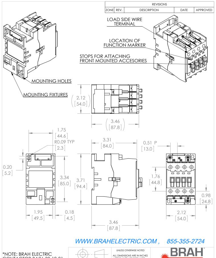
CONTACTOR BA26-30-10-81 IS AN AFTERMARKET DIRECT REPLACMENT FOR A26-30-10-81, A-LINE SERIES. SUITABLE FOR USE WITH A-LINE SERIES MOTOR CONTROL SYSTEMS
