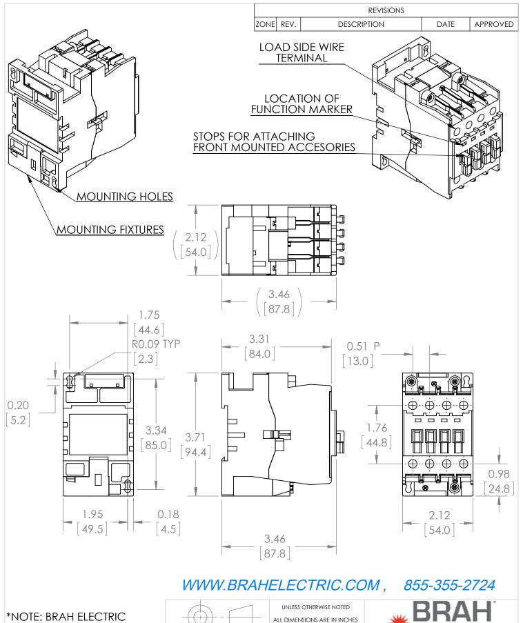
**CONTACTOR BA26-30-10-83** IS AN AFTERMARKET DIRECT REPLACMENT FOR A26-30-10-83, A-LINE SERIES. SUITABLE FOR USE WITH A-LINE SERIES MOTOR CONTROL SYSTEMS
