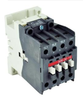
PART NUMBER – BA26-30-10-84: BRAH Electric, aftermarket direct replacement contactors for ABB A26-30-10-84, A-Line series, type A, 3P, 3PH, 28A, 600V, 10HP @ 240V, 20HP @ 480V, 25HP @ 600V, complete with 120V AC coil, and 1 N/O auxiliary contact, AC magnetic contactor, suitable for use with A-Line series motor control systems
