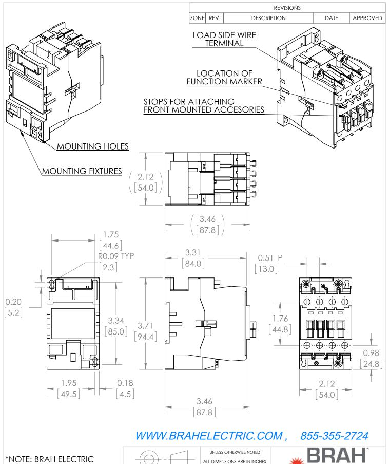
**CONTACTOR BA26-30-10-84** IS AN AFTERMARKET DIRECT REPLACMENT FOR A26-30-10-84, A-LINE SERIES. SUITABLE FOR USE WITH A-LINE SERIES MOTOR CONTROL SYSTEMS
