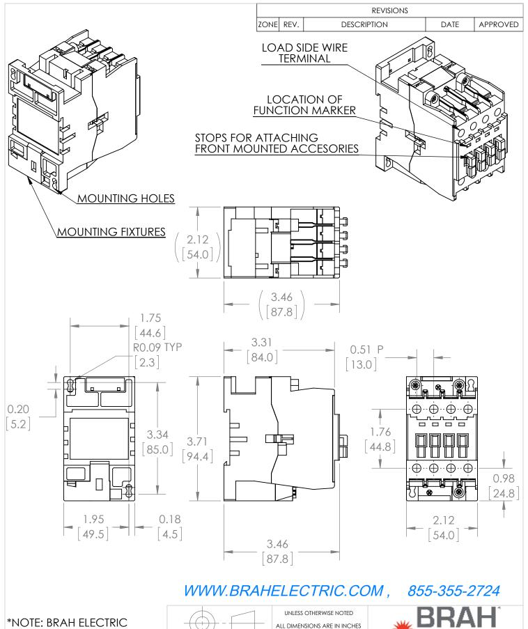
**CONTACTOR BA26-30-10-86** IS AN AFTERMARKET DIRECT REPLACMENT FOR A26-30-10-86, A-LINE SERIES. SUITABLE FOR USE WITH A-LINE SERIES MOTOR CONTROL SYSTEMS
