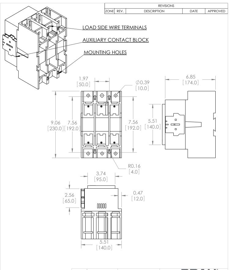
\*NOTE: BRAH ELECTRIC CONTACTOR BA260-30-11-81 IS AN AFTERMARKET DIRECT REPLACMENT FOR A260-30-11-81, A-LINE SERIES. SUITABLE FOR USE WITH A-LINE SERIES MOTOR CONTROL **SYSTEMS**
