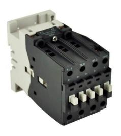
PART NUMBER – BA30-30-10-42: BRAH Electric, aftermarket direct replacement contactors for ABB A30-30-10-42 A-Line series, type A, 3P, 3PH, 34A, 600V, 10HP @ 240V, 25HP @ 480V, 30HP @ 600V, complete with 277V AC coil, and 1 N/O auxiliary contact, AC magnetic contactor, suitable for use with A-Line series motor control systems
