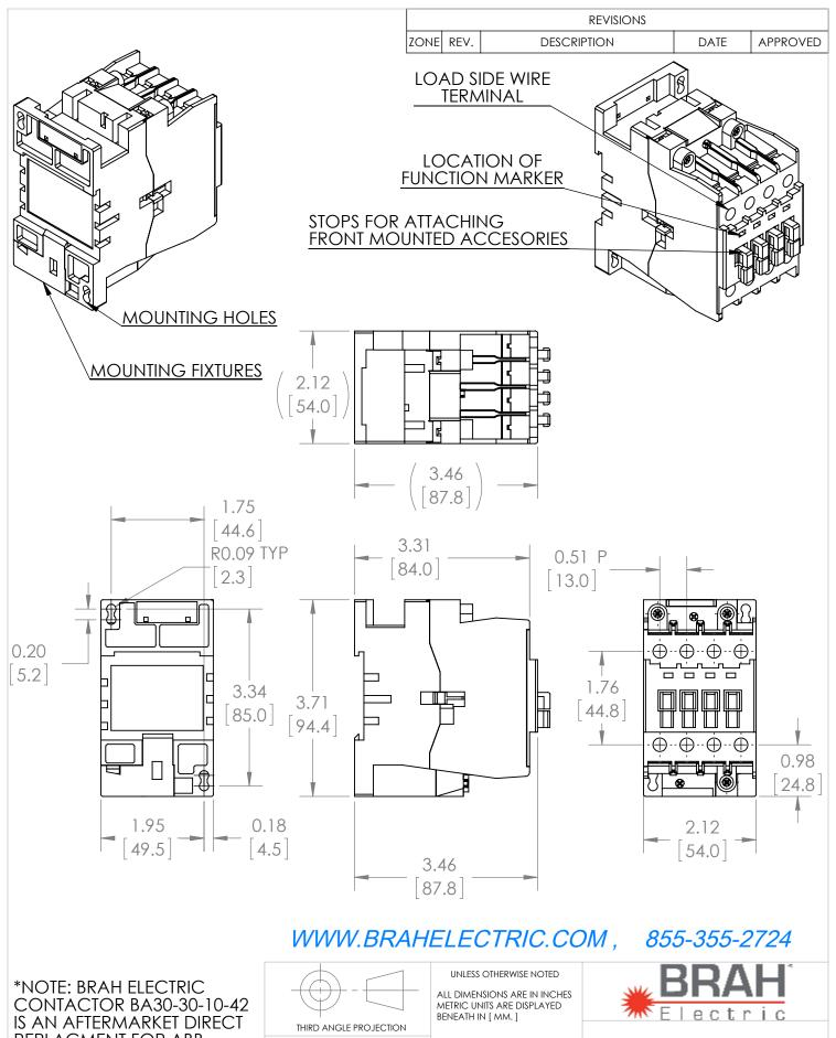
REPLACMENT FOR ABB A30-30-10-42, A-LINE SERIES. SUITABLE FOR USE WITH A-LINE SERIES MOTOR CONTROL SYSTEMS
