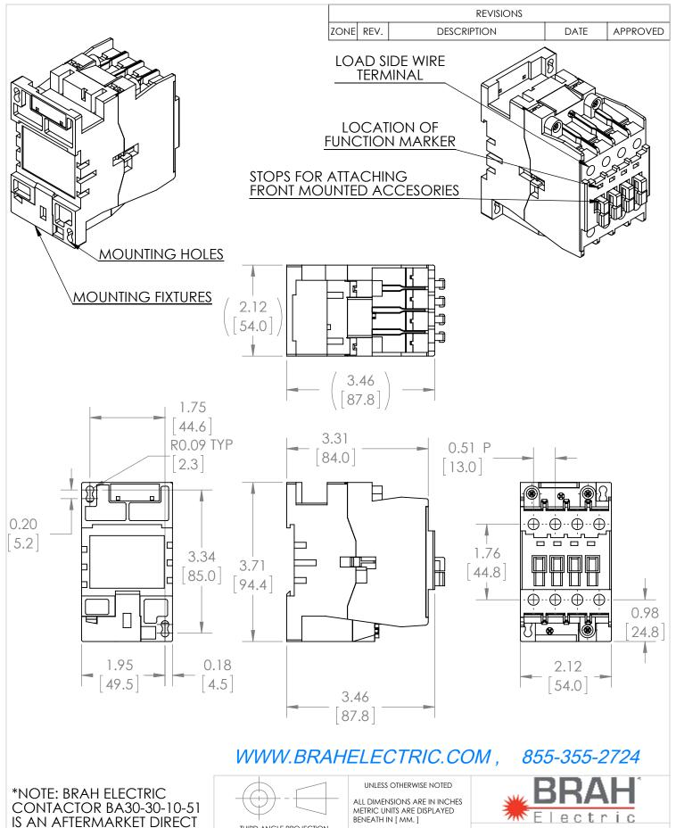
IS AN AFTERMARKET DIRECT REPLACMENT FOR ABB A30-30-10-51, A-LINE SERIES. SUITABLE FOR USE WITH A-LINE SERIES MOTOR CONTROL SYSTEMS
