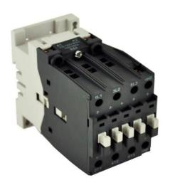
PART NUMBER – BA30-30-10-51: BRAH Electric, aftermarket direct replacement contactors for ABB A30-30-10-51, A-Line series, type A, 3P, 3PH, 34A, 600V, 10HP @ 240V, 25HP @ 480V, 30HP @ 600V, complete with 480V AC coil, and 1 N/O auxiliary contact, AC magnetic contactor, suitable for use with A-Line series motor control systems
