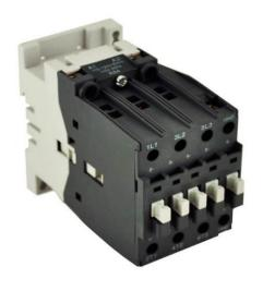
PART NUMBER – BA30-30-10-83: BRAH Electric, aftermarket direct replacement contactors for ABB A30-30-10-83, A-Line series, type A, 3P, 3PH, 34A, 600V, 10HP @ 240V, 25HP @ 480V, 30HP @ 600V, complete with 48V AC coil, and 1 N/O auxiliary contact, AC magnetic contactor, suitable for use with A-Line series motor control systems
