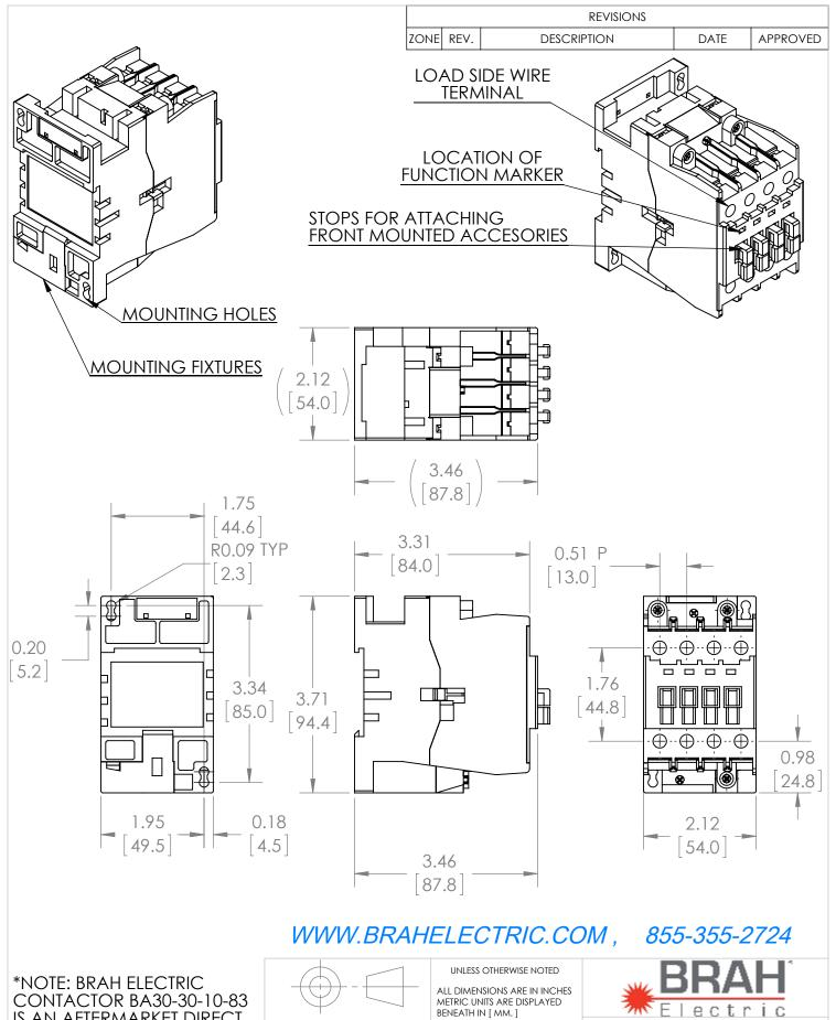
IS AN AFTERMARKET DIRECT REPLACMENT FOR ABB A30-30-10-83, A-LINE SERIES. SUITABLE FOR USE WITH A-LINE SERIES MOTOR CONTROL SYSTEMS
