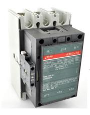
**PART NUMBER – BA300-30-11:** BRAH Electric, aftermarket direct replacement contactors for ABB A302-30-11, A-Line series, type A300, 3P, 3PH, 302A, 600V, complete with 120V AC coil, and 1 NO/1NC auxiliary contact, AC contactor, suitable for use with A-Line series motor control systems.
