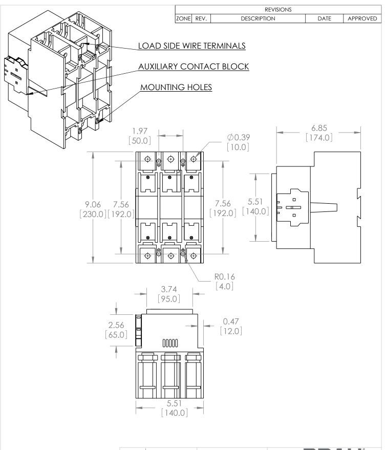
\*NOTE: BRAH ELECTRIC CONTACTOR BA300-30-11-81 IS AN AFTERMARKET DIRECT REPLACMENT FOR A300-30-11-81, A-LINE SERIES. SUITABLE FOR USE WITH A-LINE SERIES MOTOR CONTROL **SYSTEMS**
