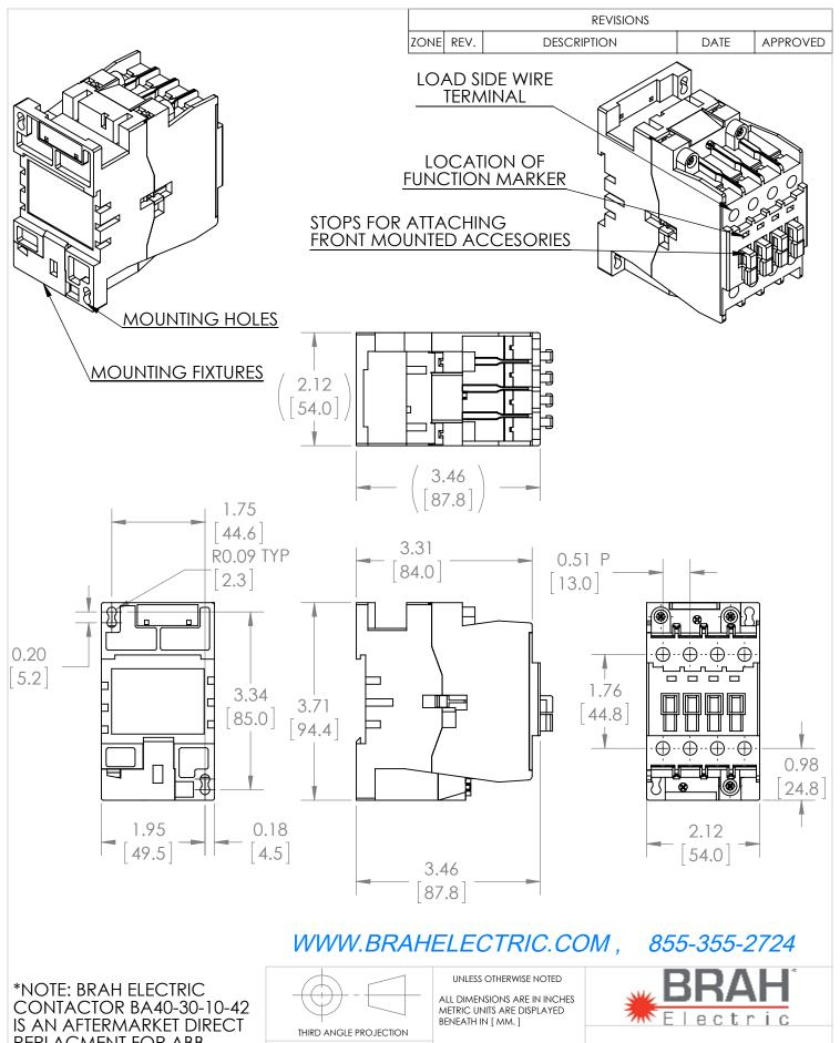
REPLACMENT FOR ABB A40-30-10-42, A-LINE SERIES. SUITABLE FOR USE WITH A-LINE SERIES MOTOR CONTROL SYSTEMS
