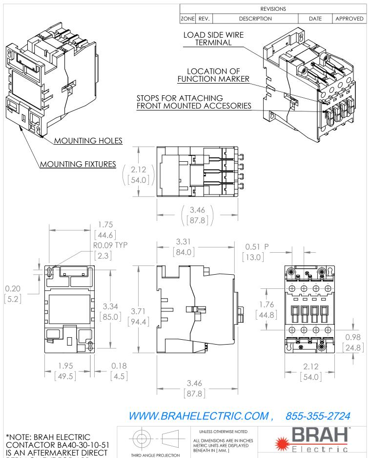
REPLACMENT FOR ABB A40-30-10-51, A-LINE SERIES. SUITABLE FOR USE WITH A-LINE SERIES MOTOR CONTROL SYSTEMS
