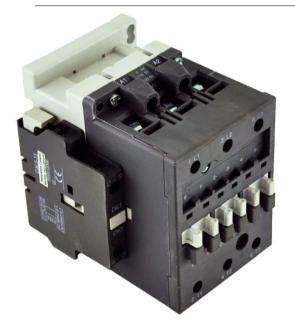
**PART NUMBER – BA63-30-11-51**: BRAH Electric, aftermarket direct replacement contactors for ABB A63-30-11-51, A-Line series, type A, 3P, 3PH, 65A, 600V, 25HP @ 240V, 50HP @ 480V, 60HP @ 600V, complete with 480V AC coil, and 1 NO/NC auxiliary contact, AC magnetic contactor, suitable for use with A-Line series motor control systems
