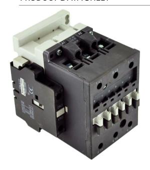
PART NUMBER – BA63-30-11-86: BRAH Electric, aftermarket direct replacement contactors for ABB A63-30-11-86, A-Line series, type A, 3P, 3PH, 65A, 600V, 25HP @ 240V, 50HP @ 480V, 60HP @ 600V, complete with 415/440V AC coil, and 1 NO/NC auxiliary contact, AC magnetic contactor, suitable for use with A-Line series motor control systems
