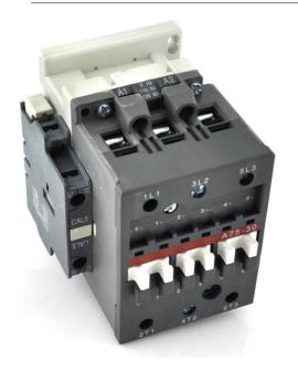
PART NUMBER – BA75-30-11-42: BRAH Electric, aftermarket direct replacement contactors for ABB A75-30-11-42, A-Line series, type A, 3P, 3PH, 80A, 600V, 30HP @ 240V, 60HP @ 480V, 75HP @ 600V, complete with 277V AC coil, and 1 NO/NC auxiliary contact, AC magnetic contactor, suitable for use with A-Line series motor control systems
