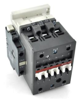
**PART NUMBER – BA75-30-11-81**: BRAH Electric, aftermarket direct replacement contactors for ABB A75-30-11-81, A-Line series, type A, 3P, 3PH, 80A, 600V, 30HP @ 240V, 60HP @ 480V, 75HP @ 600V, complete with 24V AC coil, and 1 NO/NC auxiliary contact, AC magnetic contactor, suitable for use with A-Line series motor control systems
