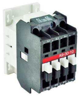
**PART NUMBER – BA9-30-10-81**: BRAH Electric, aftermarket direct replacement contactors for ABB A9-30-10-81, A-Line series, type A, 3P, 3PH, 9A, 600V, 2HP @ 24V, 5HP @ 480V, 7.5HP @ 600V, complete with 24V AC coil, and 1 N/O auxiliary contact, AC magnetic contactor, suitable for use with A-Line series motor control systems
