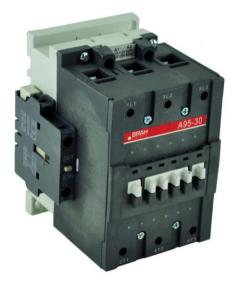
**PART NUMBER – BA95-30-11-42**: BRAH Electric, aftermarket direct replacement contactors for ABB A95-30-11-42, A-Line series, type A, 3P, 3PH, 95A, 600V, 30HP @ 240V, 60HP @ 480V, 75HP @ 600V, complete with 277V AC coil, and 1 N/O - 1 N/C auxiliary contact, AC magnetic contactor, suitable for use with A-Line series motor control systems
