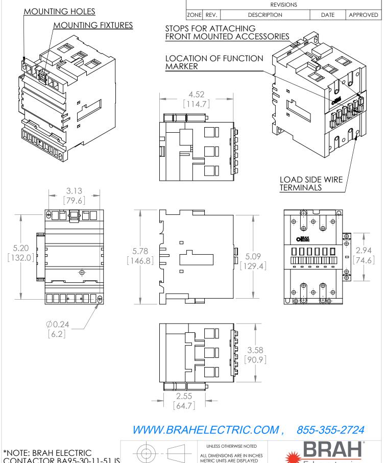
CONTACTOR BA95-30-11-51 IS AN AFTERMARKET DIRECT REPLACMENT FOR A95-30-11-51, A-LINE SERIES. SUITABLE FOR USE WITH A-LINE SERIES MOTOR CONTROL SYSTEMS
