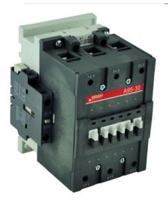
PART NUMBER – BA95-30-11-55: BRAH Electric, aftermarket direct replacement contactors for ABB A95-30-11-55, A-Line series, type A, 3P, 3PH, 95A, 600V, 30HP @ 240V, 60HP @ 480V, 75HP @ 600V, complete with 500/600V AC coil, and 1 N/O - 1 N/C auxiliary contact, AC magnetic contactor, suitable for use with A-Line series motor control systems
