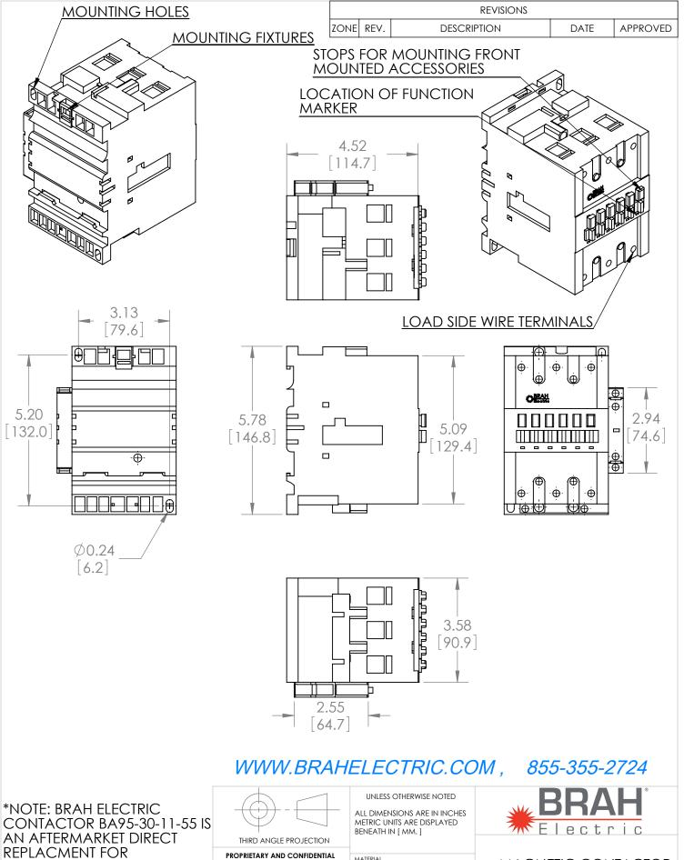
CONTACTOR BA95-30-11-55 IS AN AFTERMARKET DIRECT REPLACMENT FOR A95-30-11-55,A-LINE SERIES. SUITABLE FOR USE WITH A-LINE SERIES MOTOR CONTROL SYSTEMS
