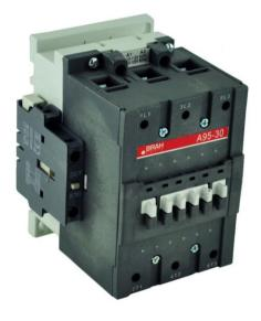
**PART NUMBER – BA95-30-11-86**: BRAH Electric, aftermarket direct replacement contactors for ABB A95-30-11-86, A-Line series, type A, 3P, 3PH, 95A, 600V, 30HP @ 240V, 60HP @ 480V, 75HP @ 600V, complete with 415/440V AC coil, and 1 N/O - 1 N/C auxiliary contact, AC magnetic contactor, suitable for use with A-Line series motor control systems
