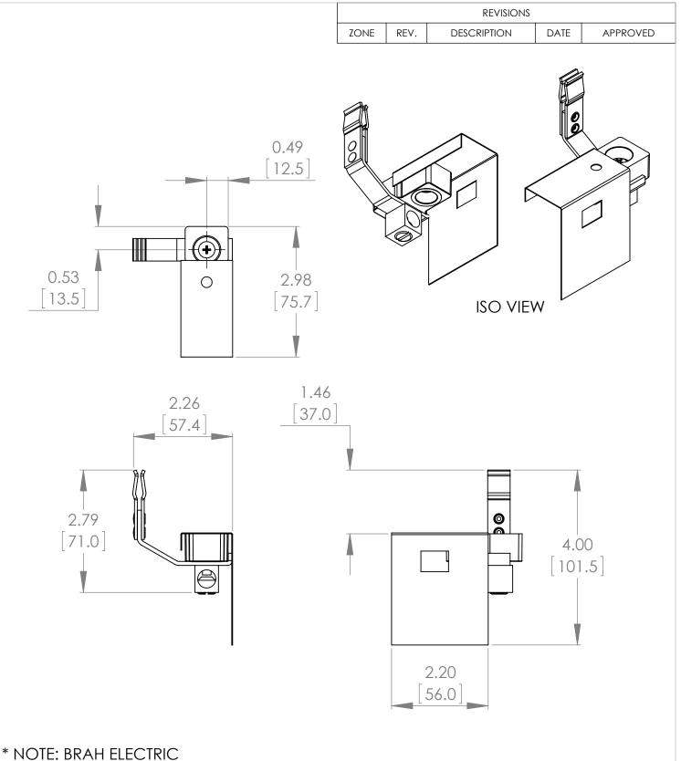
\* NOTE: BRAH ELECTRIC NEUTRAL KITS ARE A DIRECT REPLACEMENT FOR GENERAL ELECTRIC, DH SERIES, NEUTRAL KITS, NEUTRAL KIT ASSEMBLY, RATED FOR 30A-100A, 600V; SUITABLE FOR USE WITH 30A - 100A 600V RATED TYPE DH FUSIBLE BUS PLUGS
