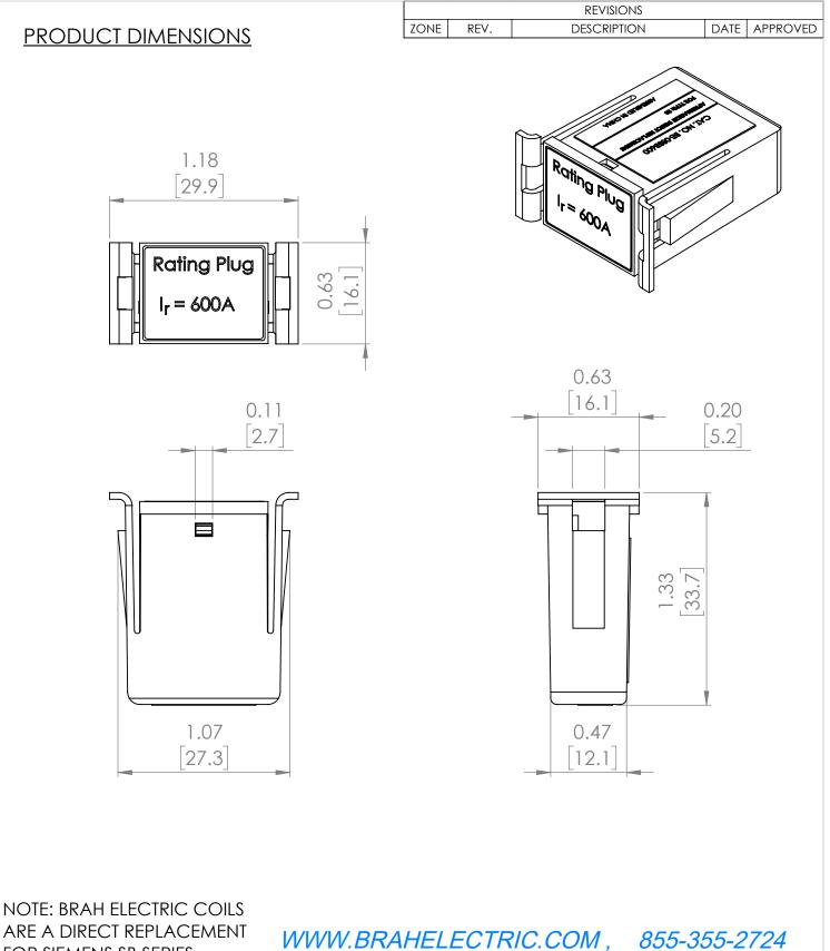
ARE A DIRECT REPLACEMENT FOR SIEMENS SB SERIES, 600 AMP RATING PLUG, TYPE 08SB, SUITABLE FOR SIEMENS SB SERIES 800 AMP INSULATED FRAME TYPES SBA, SBH, SBS EQUIPPED WITH SB-EC or TL SERIES SOLID STATE ELCTRONIC TRIP UNITS.
