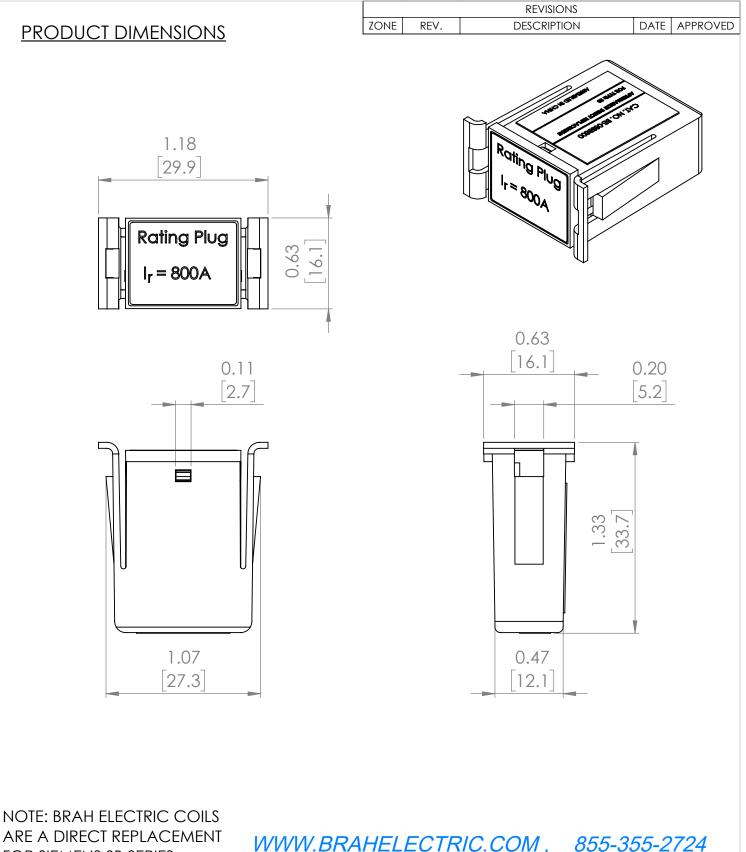
ARE A DIRECT REPLACEMENT FOR SIEMENS SB SERIES, 800 AMP RATING PLUG, TYPE **08SB, SUITABLE FOR SIEMENS** SB SERIES 800 AMP INSULATED FRAME TYPES SBA, SBH, SBS EQUIPPED WITH SB-EC or TL SERIES SOLID STATE ELCTRONIC TRIP UNITS.
