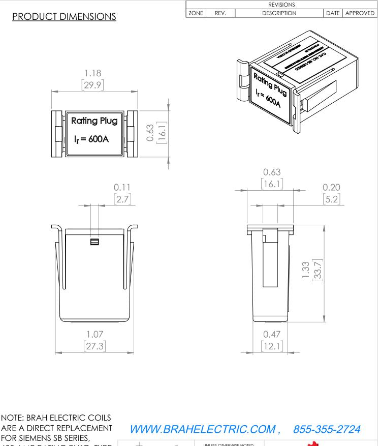
FOR SIEMENS SB SERIES, 600 AMP RATING PLUG, TYPE 12SB, SUITABLE FOR SIEMENS SB SERIES 1200 AMP INSULATED FRAME TYPES SBA, SBH, SBS EQUIPPED WITH SB-EC or TL SERIES SOLID STATE ELCTRONIC TRIP UNITS.
