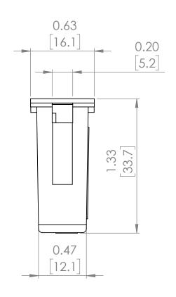
NOTE: BRAH ELECTRIC COILS ARE A DIRECT REPLACEMENT FOR SIEMENS SB SERIES, 1200 AMP RATING PLUG, TYPE 16SB, SUITABLE FOR SIEMENS SB SERIES 1600 AMP INSULATED FRAME TYPES SBA, SBH, SBS EQUIPPED WITH SB-EC or TL SERIES SOLID STATE ELCTRONIC TRIP UNITS.
