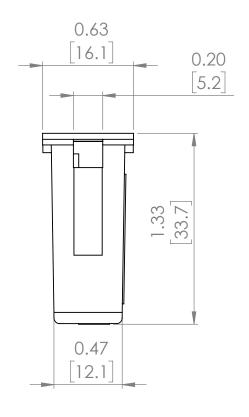
NOTE: BRAH ELECTRIC COILS ARE A DIRECT REPLACEMENT FOR SIEMENS SB SERIES, 1600 AMP RATING PLUG, TYPE 32SB, SUITABLE FOR SIEMENS SB SERIES 3200 AMP INSULATED FRAME TYPES SBA, SBH, SBS EQUIPPED WITH SB-EC or TL SERIES SOLID STATE ELCTRONIC TRIP UNITS.
