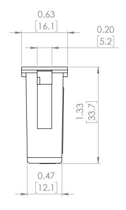
NOTE: BRAH ELECTRIC COILS ARE A DIRECT REPLACEMENT FOR SIEMENS SB SERIES, 2000 AMP RATING PLUG, TYPE 40SB, SUITABLE FOR SIEMENS SB SERIES 4000 AMP INSULATED FRAME TYPES SBA, SBH, SBS EQUIPPED WITH SB-EC or TL SERIES SOLID STATE ELCTRONIC TRIP UNITS.
