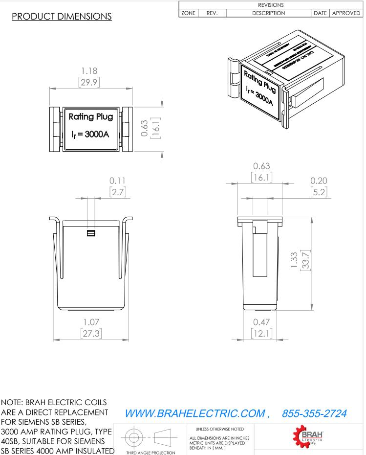
SB SERIES 4000 AMP INSULATED FRAME TYPES SBA, SBH, SBS EQUIPPED WITH SB-EC or TL SERIES SOLID STATE ELCTRONIC TRIP UNITS.
