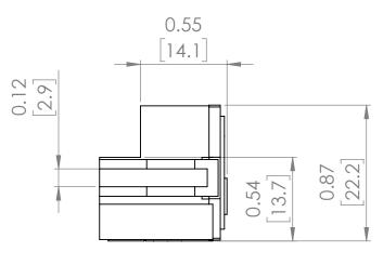
NOTE: BRAH ELECTRIC COILS ARE A DIRECT REPLACEMENT FOR GENERAL ELECTRIC, POWER BREAK 1, TYPE TR10,600 Amp PLUG FOR 1000 Amp CT SENSOR RATING, SUITABLE FOR USE WITH ALL TP, TC, THP, THC EQUIPPED WITH MICROVERSA TRIP RMS-9 SOLID STATE ELECTRONIC
