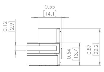
NOTE: BRAH ELECTRIC **COILS ARE A DIRECT** REPLACEMENT FOR GENERAL ELECTRIC, POWER BREAK 1, TYPE TR16,1200 Amp PLUG FOR 1600 Amp CT SENSOR RATING, SUITABLE FOR USE WITH ALL TP, TC, THP, THC, AKR50, AKR50H EQUIPPED WITH MICROVERSA TRIP RMS-9 SOLID STATE ELECTRONIC TRIP UNITS.
